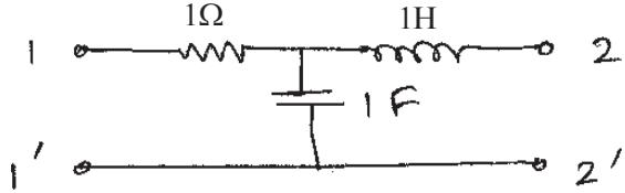
d) Find R, L, C and G in the following circuit while impedance
