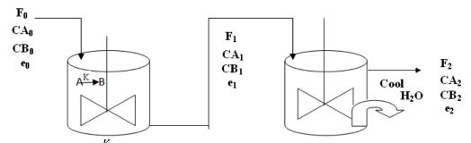
A reaction  $A \xrightarrow{K} B$  takes place in a perfectly mixed CSTR. In order to prevent the formation of excess of B the contents of CSTR are sent into a  $2^{nd}$  CSTR where the reaction fluid is quenched by supplying cooling water inside a coil which will remove the heat of reaction.
