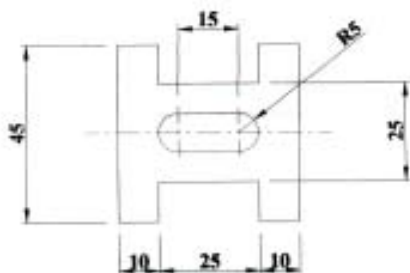
Fig. 1 Material: Al, 1mm thick
