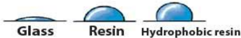
Fig. 1 Shape of waterdrops on the surfaces of glass, resin and hydrophobic resin
